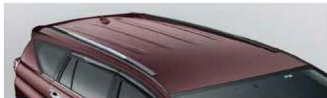
#2622-INV-16 ROOF SIDE BAR , ABS BLOW , W/ ALUM MOULDING
